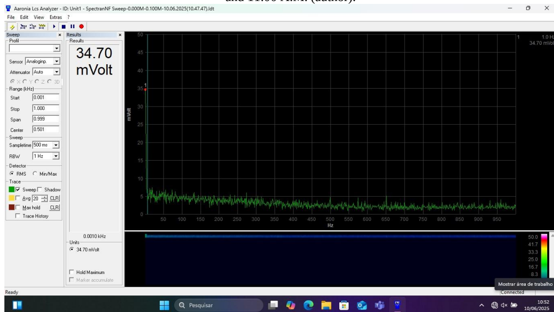
Figure 4 - Voltage curve in mV versus frequency from 1 Hz to 1000 Hz on June 10, 2025, at ITA between 10:00 and 11:00 A.M. (author).
