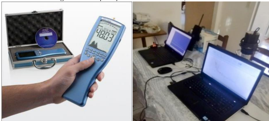
Figure 1 - View of the Spectran NF-5035 detector, used in this work.
